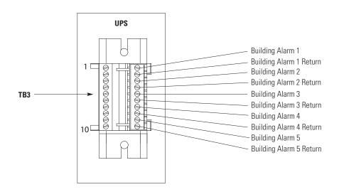
**NOTE** All building alarm inputs require an isolated normally-open or normally-closed contact or switch (rated at 24 Vdc, 20 mA minimum) connected between the alarm input and common terminal as shown. Building alarm inputs can be programmed for use with either normally-open or normally-closed contacts. All control wiring and relay and switch contacts are customer-supplied.
