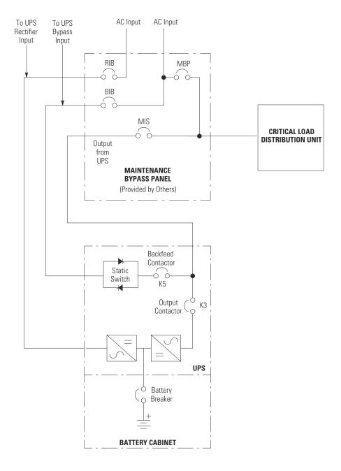
RIB: Rectifier Input Breaker
