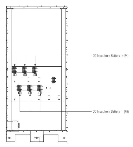
Figure 4-10. UPS Power Terminal Detail BB – Common Battery
