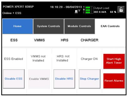
Figure 7-40. Energy Advantage Architecture (EAA) Screen
