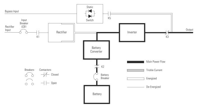
**NOTE** On a UPS configured as an IOM, the bypass input, static switch, and K5 are not present.
