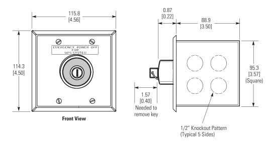
Figure 3-7. Remote EPO Switch Dimensions
