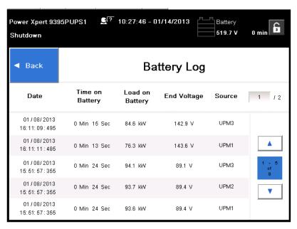
Figure 7-28. Battery Log Detail
