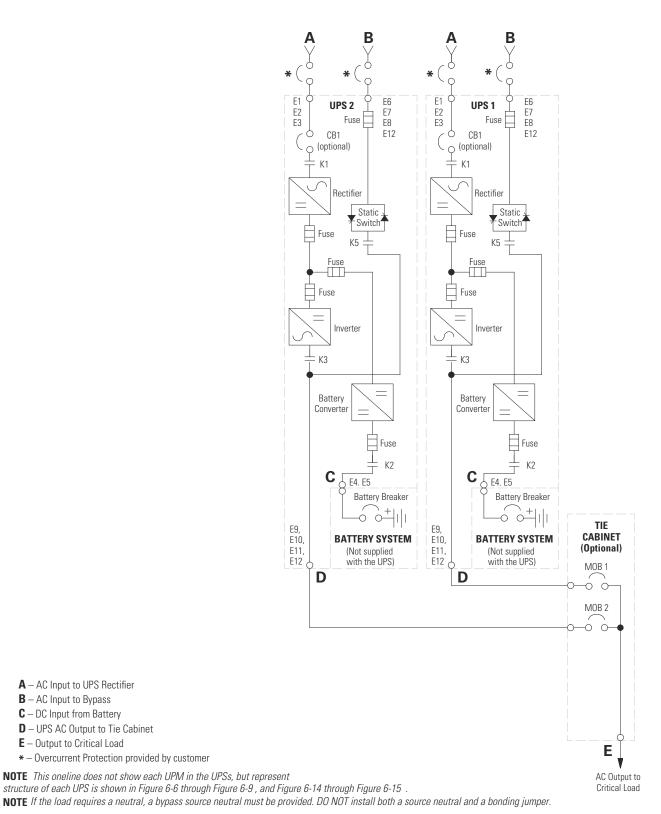
Figure 6-22. Typical Distributed Bypass System (1+1 and 2+0 Configurations)
