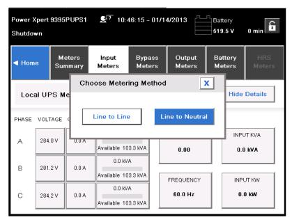
Figure 7-36. Online Mode Metering Method Option Screen
