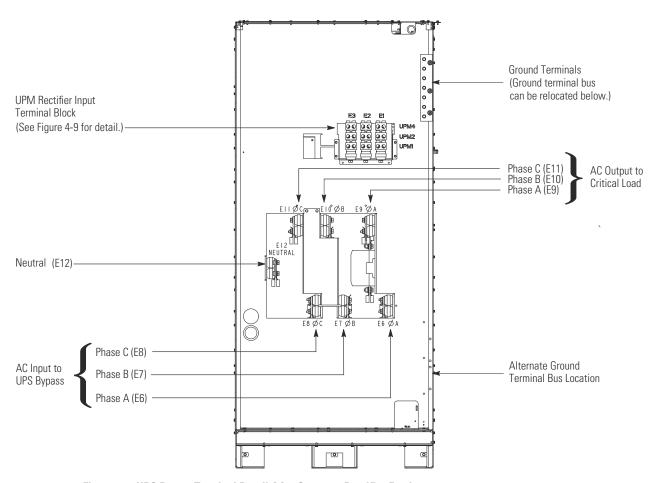
Figure 4-8. UPS Power Terminal Detail AA – Separate Rectifier Feed
