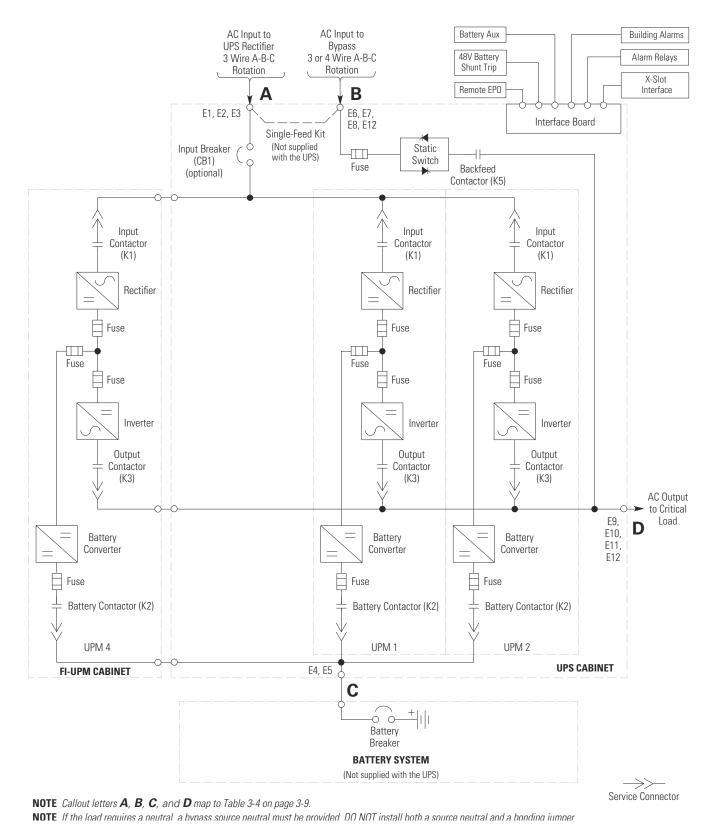
Figure 6-8. Plus 1 UPS System – Three UPM, Common Rectifier Feed, Common Battery, Dual-Feed Configuration
