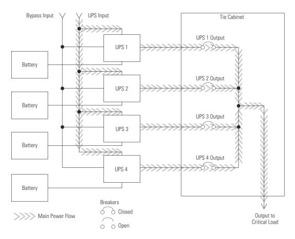
Figure 6-19. Path of Current through the UPSs in Online Mode – Distributed Bypass
