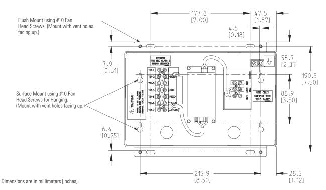
Figure 5-12. Remote Monitor Panel II Dimensions
