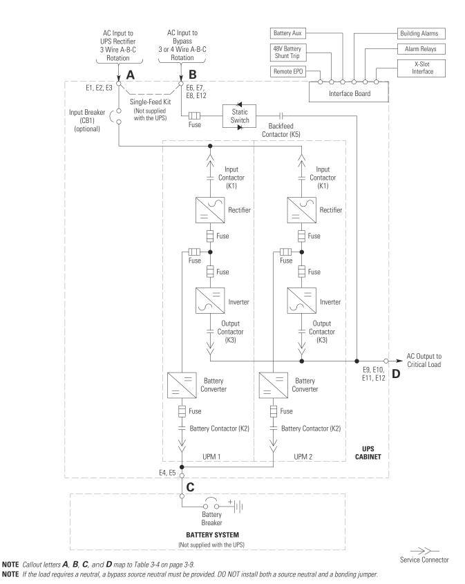
Figure 6-6. UPS System – Two UPM, Common Rectifier Feed, Common Battery, Dual-Feed Configuration
