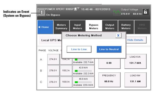
Figure 7-37. Bypass Mode Metering Method Option Screen
