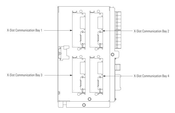
Figure 4-18. X-Slot Communication Bays
