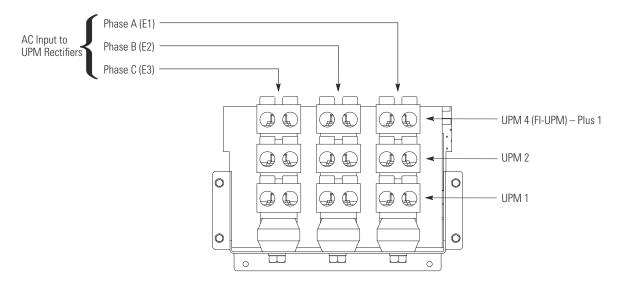
Figure 4-9. UPM Rectifier Input Power Terminal Block Detail
