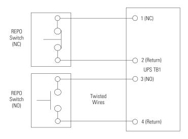
OTE REPO switch rating is 24 Vdc, 1A minimum.
