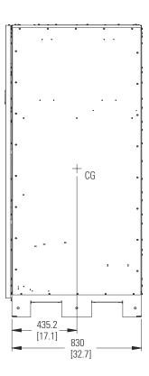
Figure 3-6. UPS Cabinet Center of Gravity
