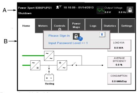
Figure 7-11. Parts of the Touch Screen
