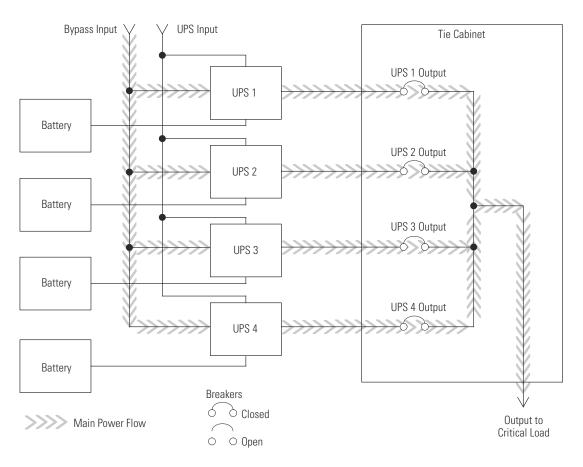
Figure 6-20. Path of Current through the UPSs in Bypass Mode – Distributed Bypass
