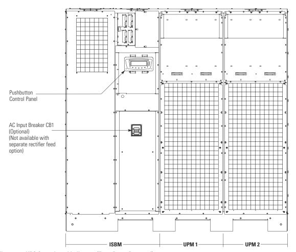
Figure 7-1. UPS Controls and Indicators (Front Doors Removed)
