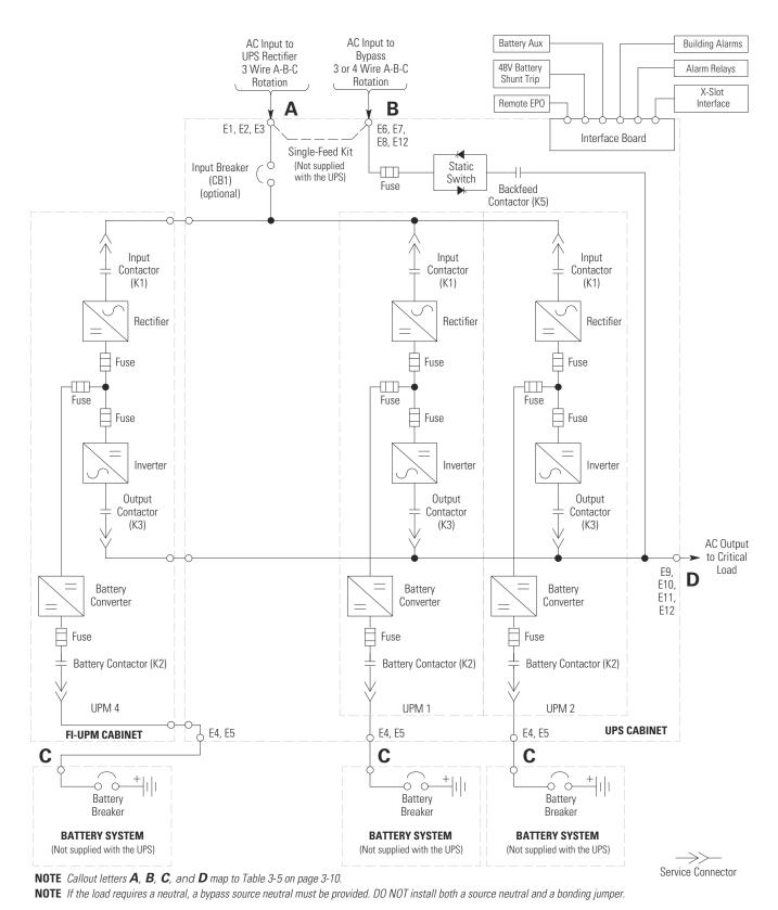
Figure 6-9. Plus 1 UPS System – Three UPM, Common Rectifier Feed, Separate Battery, Dual-Feed Configuration
