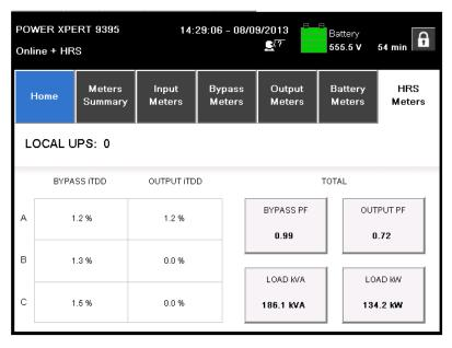
Figure 7-42. HRS Metering Screen
