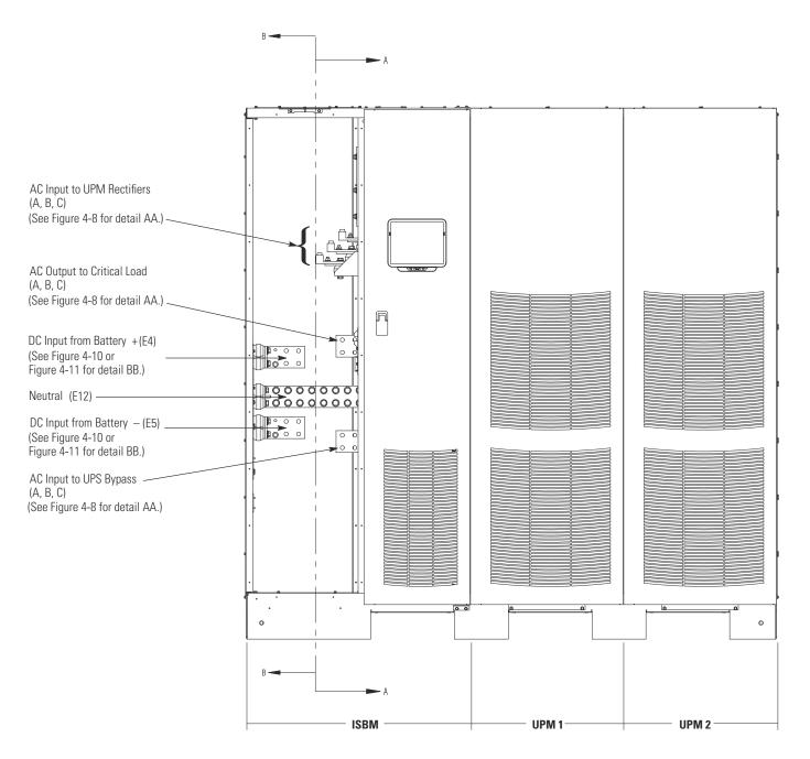
Figure 4-7. UPS Power Terminal Locations – Separate Rectifier Feed
