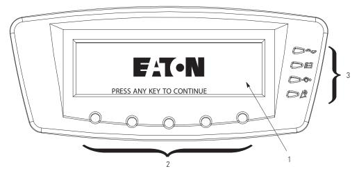
Figure 7-2. UPS Control Panel
