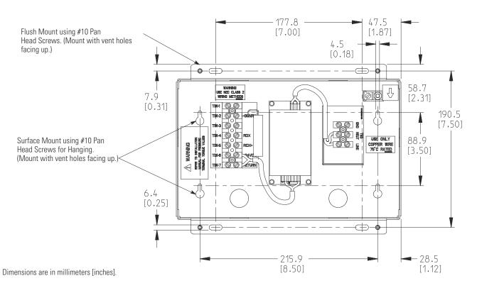
Figure 5-13. Relay Interface Module II Dimensions
