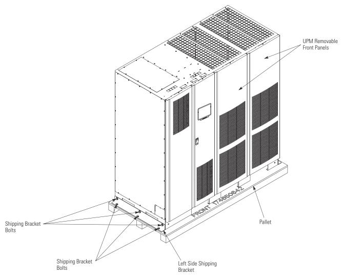
Figure 4-1. Removing the Left Side Shipping Bracket
