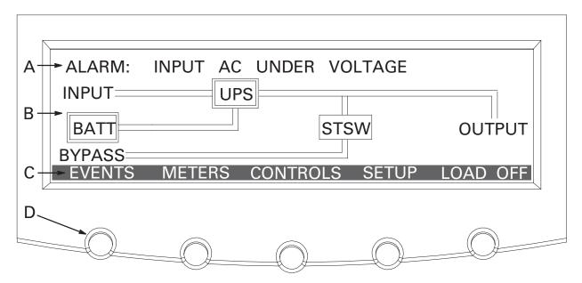
Figure 7-3. Parts of the LCD
