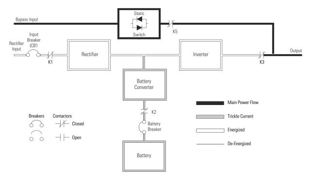
Figure 6-3. Path of Current Through the UPS in Energy Saver Mode
