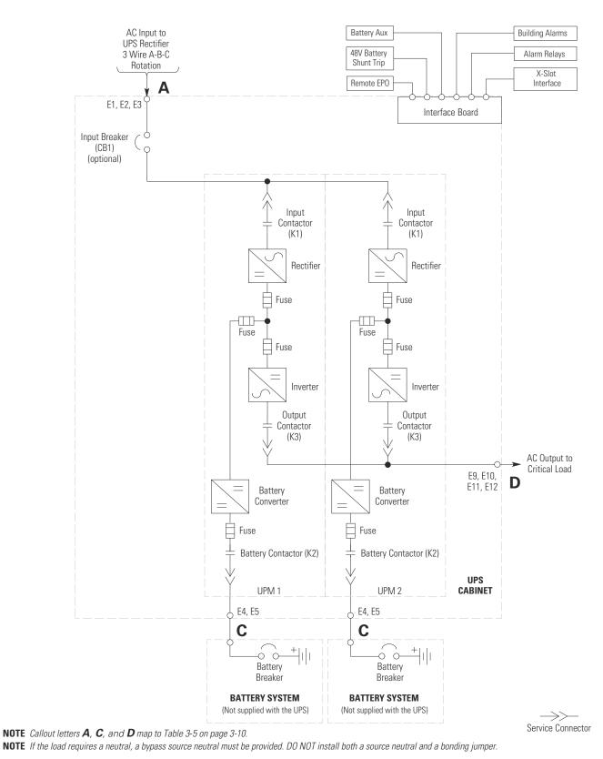
Figure 6-11. UPS System - Two UPM, Common Rectifier Feed, Separate Battery, IOM Configuration
