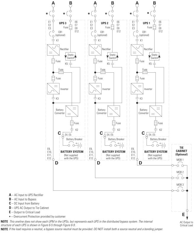
Figure 6-23. Typical Distributed Bypass System (2+1 and 3+0 Configurations)
