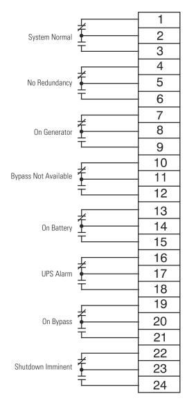
Figure 5-11. Supervisory Contact Module II TB2
