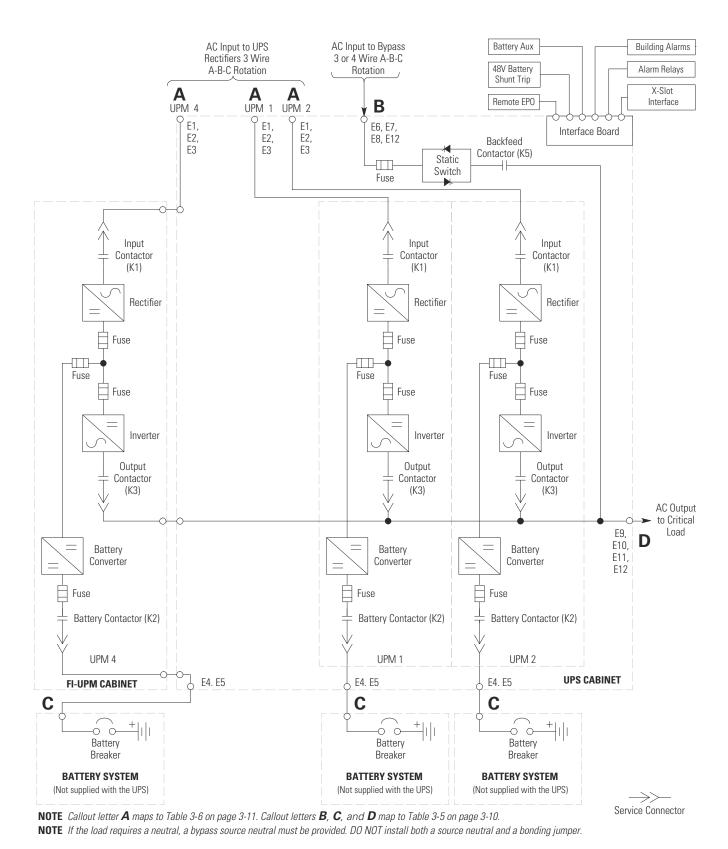
Figure 6-15. Plus 1 UPS System – Three UPM, Separate Rectifier Feed, Separate Battery, Dual-Feed Configuration
