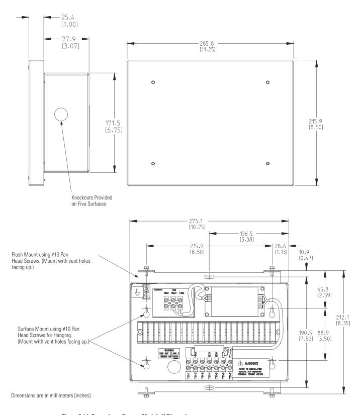
Figure 5-14. Supervisory Contact Module II Dimensions
