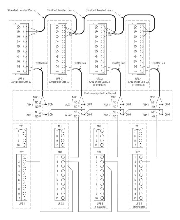
NOTE NC and NO designations on MOB AUX contacts are defined with breaker in OFF (open) position.
