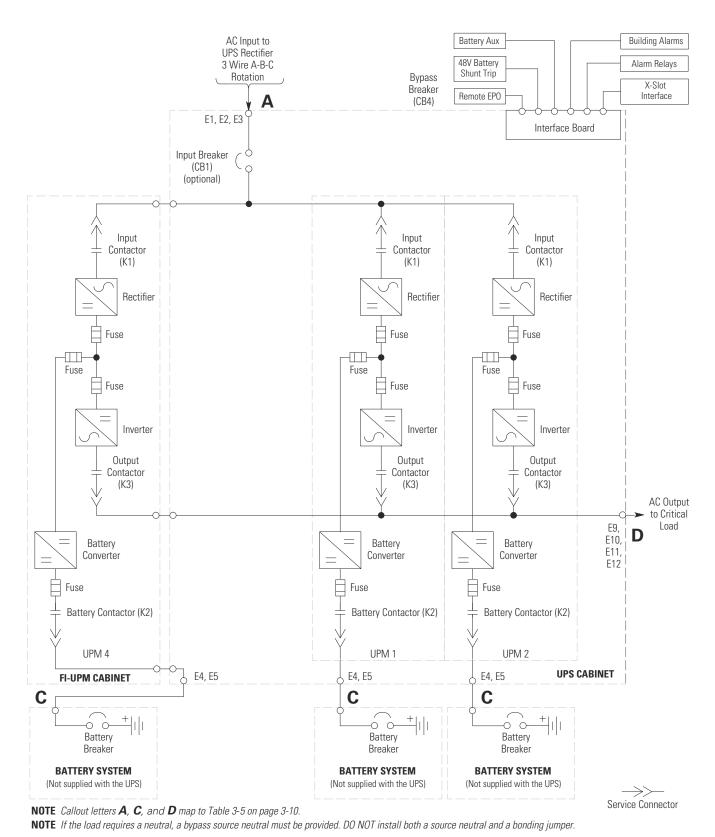
Figure 6-13. Plus 1 UPS System – Three UPM, Common Rectifier Feed, Separate Battery, IOM Configuration
