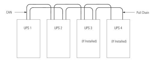
NOTE This drawing is for distributed bypass wiring purposes and is not a floor layout plan. UPSs can be placed in any physical order.
