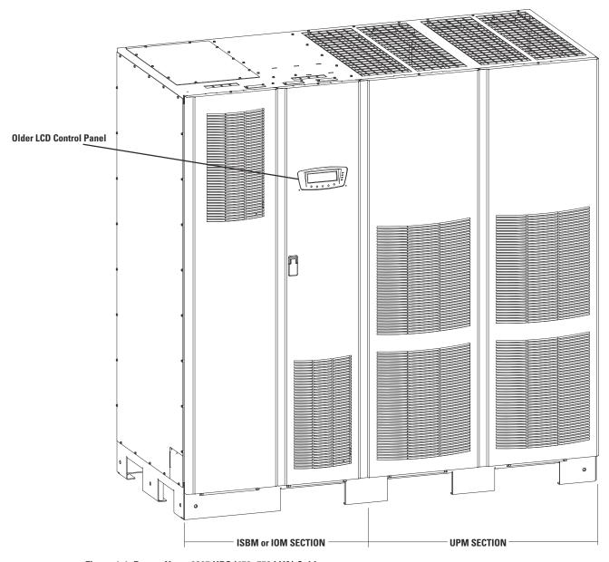
Figure 1-1. Power Xpert 9395 UPS (450-550 kVA) Cabinet
