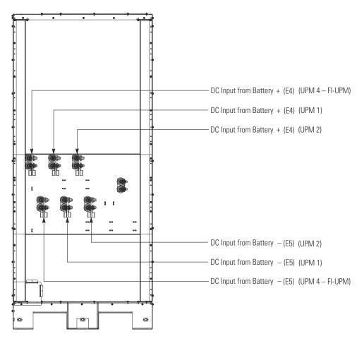
Figure 4-11. UPS Power Terminal Detail BB – Separate Battery
