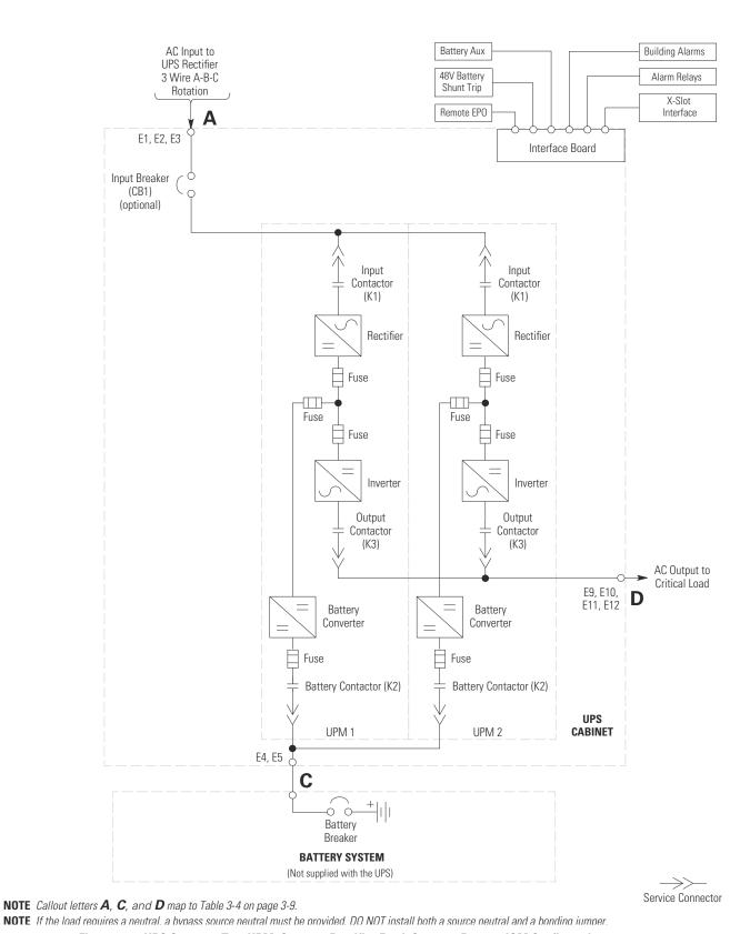
Figure 6-10. UPS System – Two UPM, Common Rectifier Feed, Common Battery, IOM Configuration
