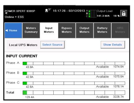
Figure 7-21. Input Meters Screen
