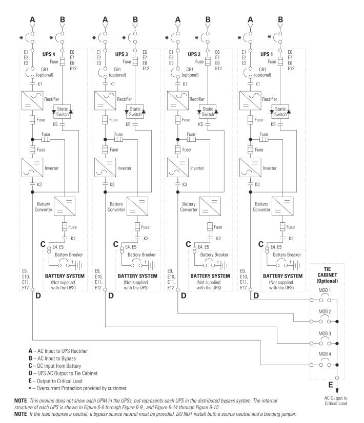
Figure 6-24. Typical Distributed Bypass System (3+1 and 4+0 Configurations)
