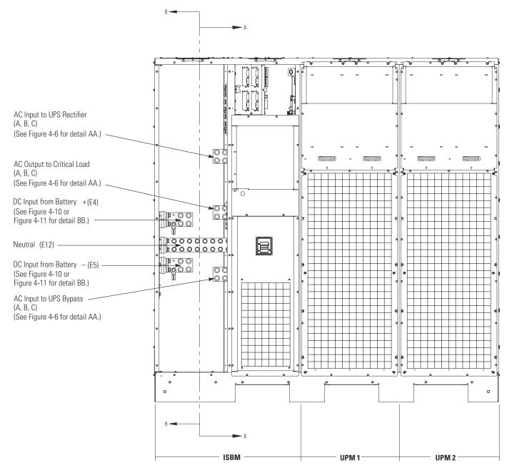
Figure 4-5. UPS Power Terminal Locations – Common Rectifier Feed
