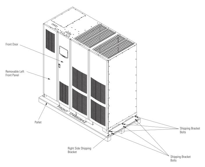
Figure 4-2. Removing the Right Side Shipping Bracket
