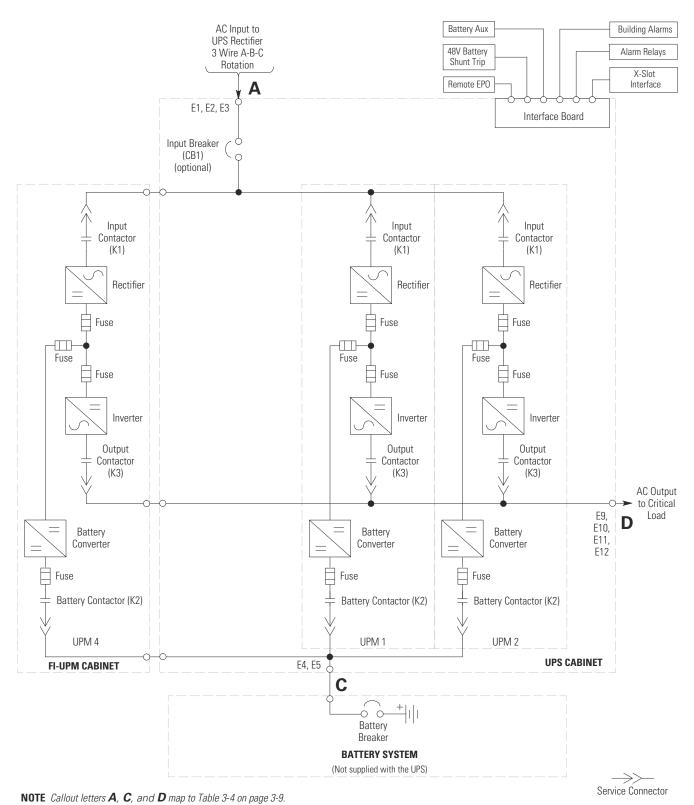
NOTE If the load requires a neutral, a bypass source neutral must be provided. DO NOT install both a source neutral and a bonding jumper.
