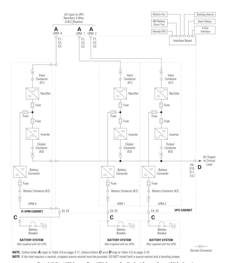
Figure 6-17. Plus 1 UPS System – Three UPM, Separate Rectifier Feed, Separate Battery, IOM Configuration
