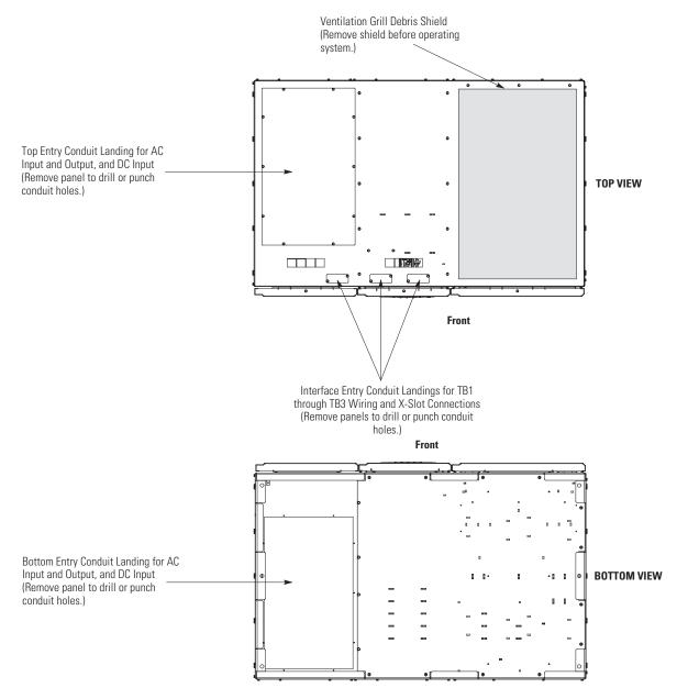
Figure 4-4. Conduit and Wire Entry Locations
