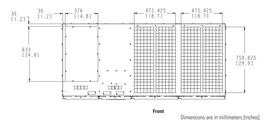
Figure 3-3. UPS Cabinet Dimensions (Top View)
