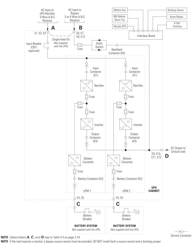
Figure 6-7. UPS System – Two UPM, Common Rectifier Feed, Separate Battery, Dual-Feed Configuration
