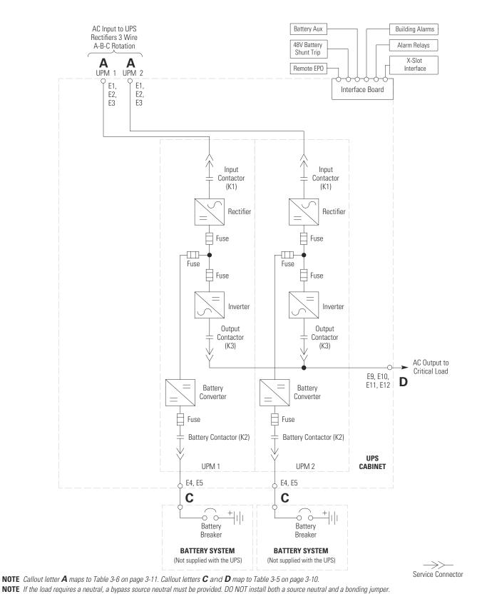
Figure 6-16. UPS System – Two UPM, Separate Rectifier Feed, Separate Battery, IOM Configuration
