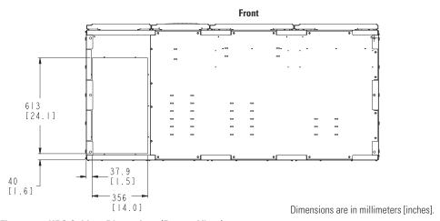
Figure 3-4. UPS Cabinet Dimensions (Bottom View)
