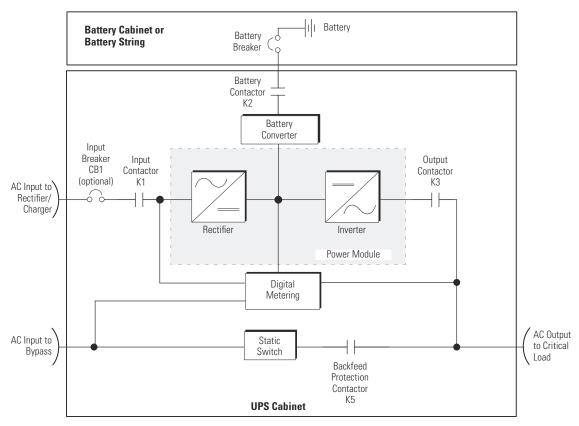
NOTE On a UPS configured as an Input Output Module (IOM), the bypass input, static switch, and backfeed protection contactor (K5) are not present.
