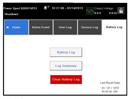
Figure 7-27. Battery Log Screen
