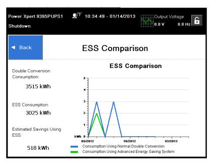
Figure 7-46. ESS Comparison Screen
