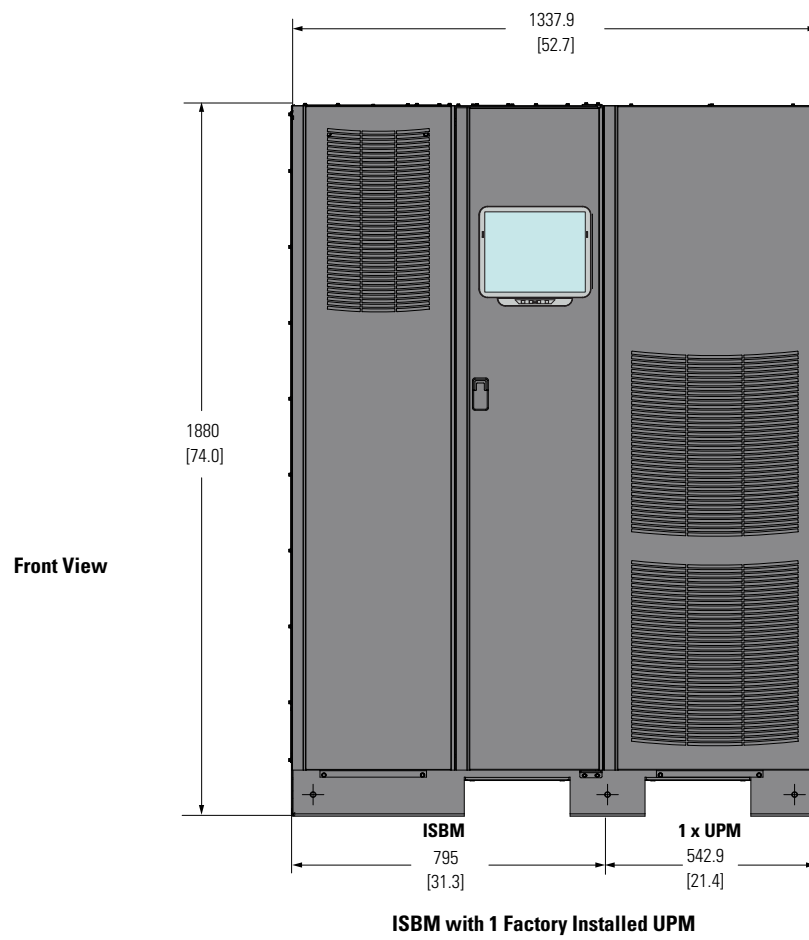
Figure 3. Single UPM Configuration Dimensions
