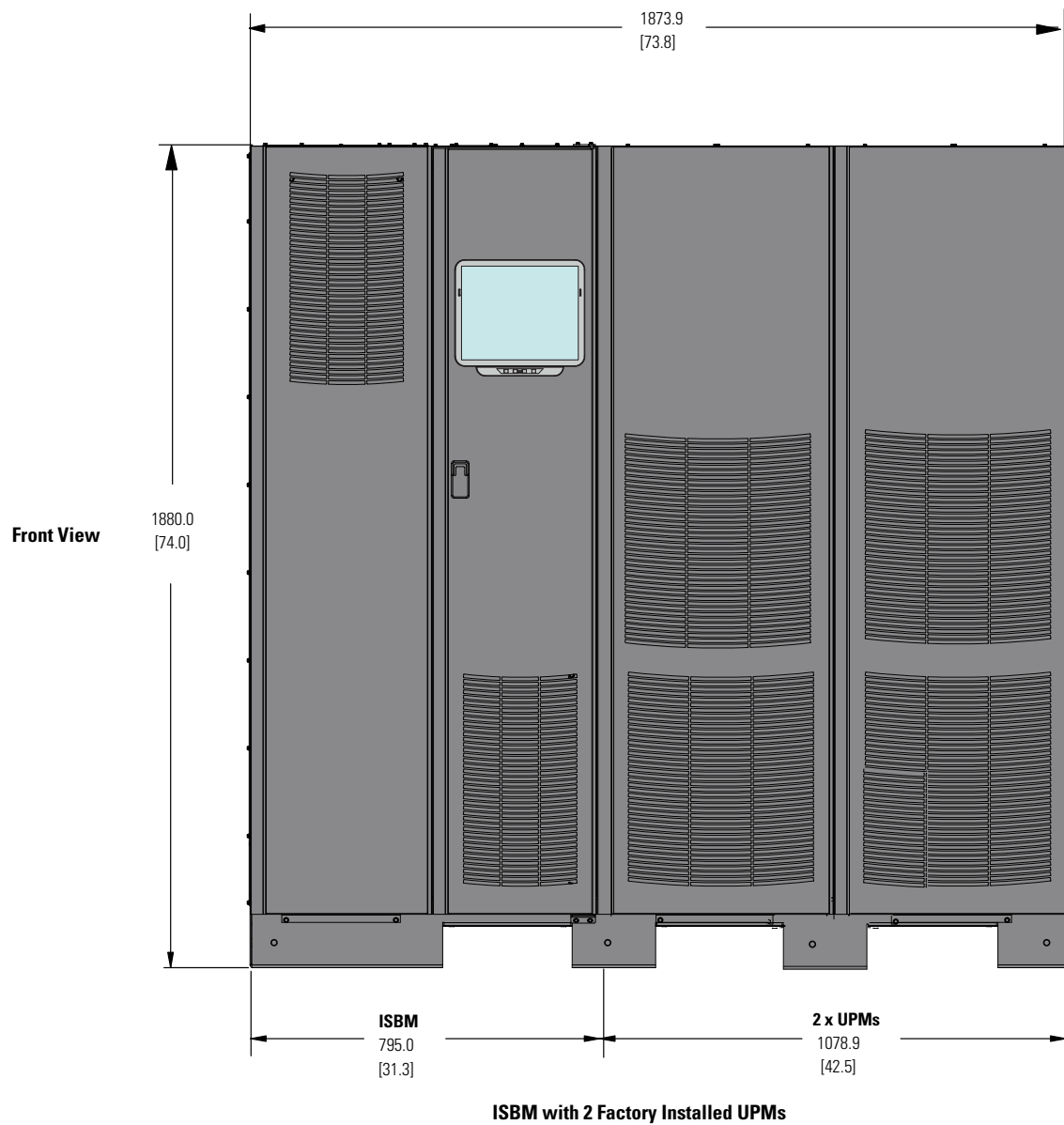
Figure 7. Two UPM Configuration Dimensions
