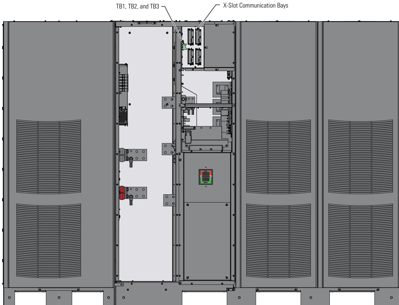
Figure 21. ISBM Section Interface Terminal Locations
