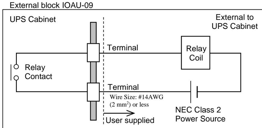
**Figure 4-20 Control Wiring for Aux Output Contacts**
