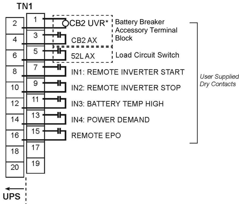
**NOTE:** For multiple battery cabinets, the UVR signals must be connected in parallel with UPS TN1-1 &-2.
