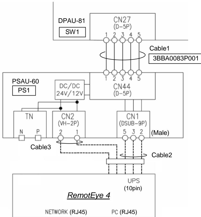
**Figure 4-24 Connection between Display Control PCB (SW1) and RemotEye® Module**
