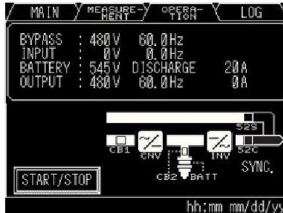
**Figure 5-21 Close Battery Breaker**
