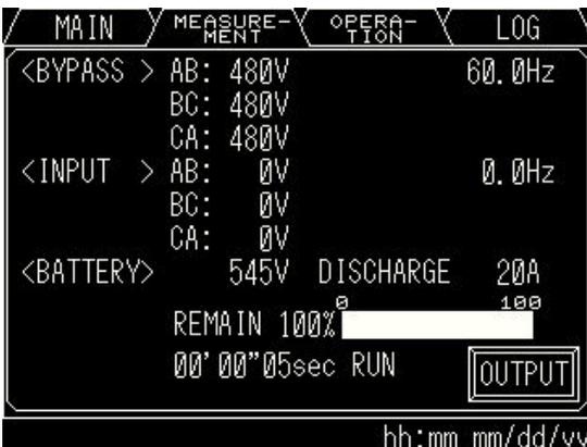
Figure 4-7 Battery Operation Values
