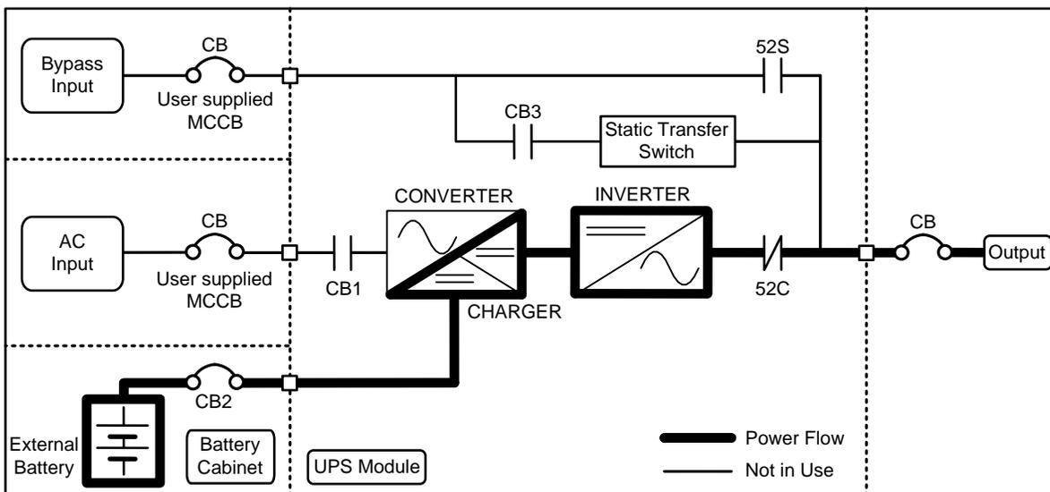
**Figure 3-3 Single Line Diagram – Battery Operation**
