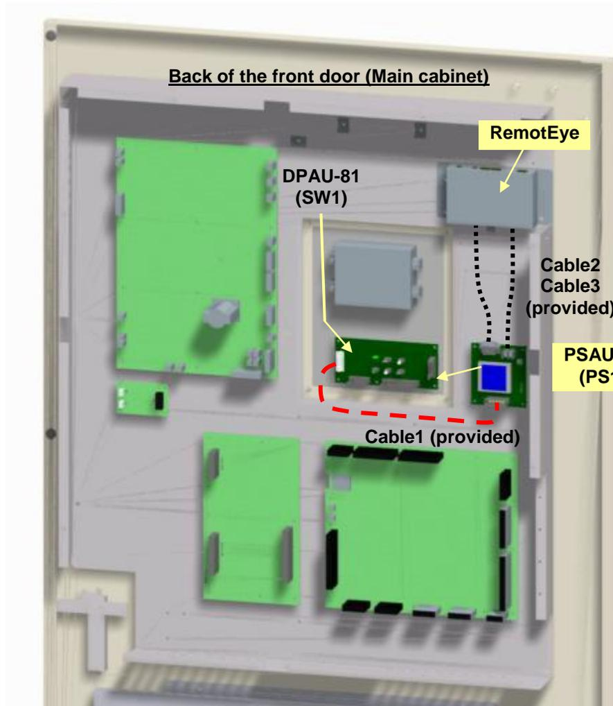
**Figure 4-22 RemotEye® Installation (Overview 300kVA)**
