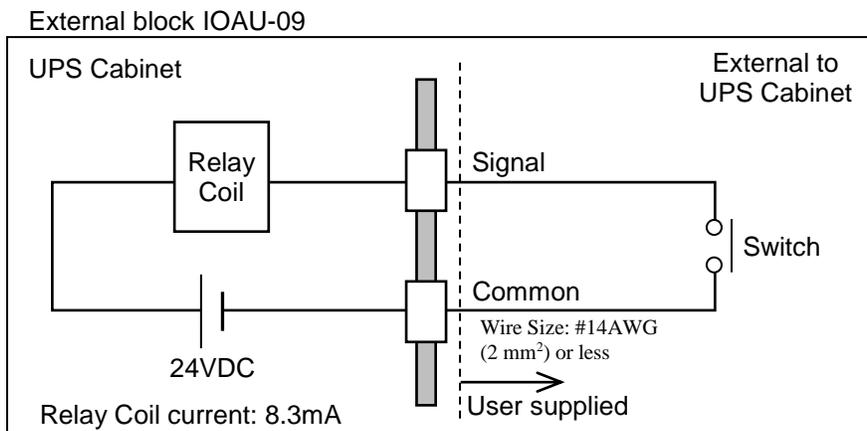
**Figure 4-18 Control Wiring for Aux Input Contacts**
