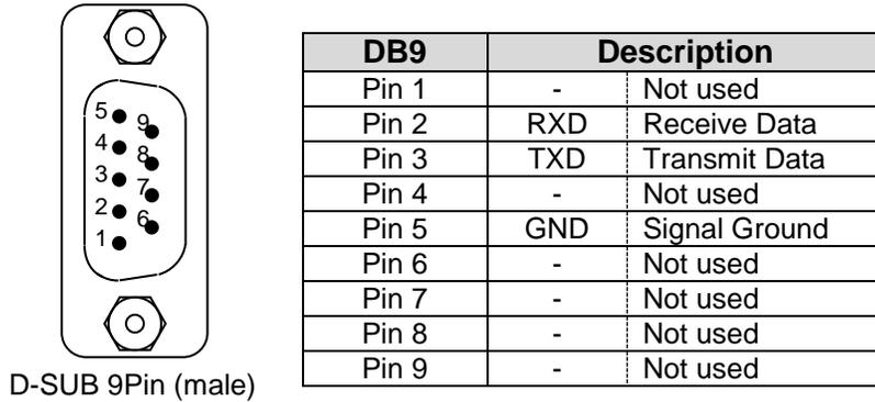
Figure 4-28 Connector (CN1) of PSAU-60 (PS1)
