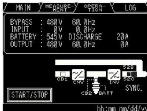
**Figure 5-26 UPS Transfers to Bypass**
