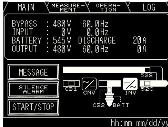
**Figure 4-16 Main screen (Fault indication)**
