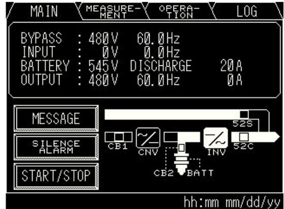
Figure 4-15 Measurement screen (Battery Operation)
