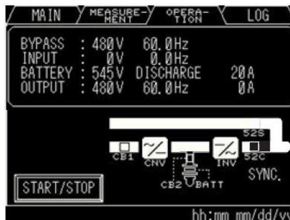
**Figure 5-27 Open Battery Breaker**
