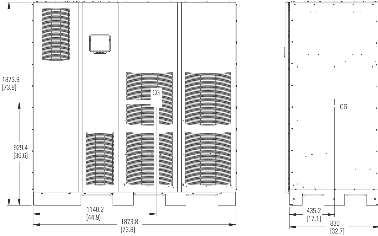
Figure 3-6. UPS Cabinet Center of Gravity
