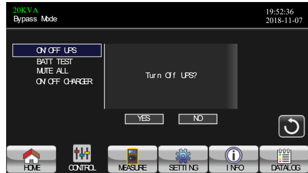
TURN OFF UPS
