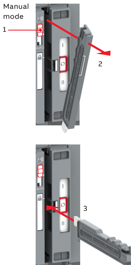
Fig. 3.3 Mounting of the handle in the operating position
