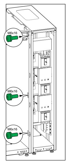
8. Lower the front and rear leveling feet on the UPS and the maintenance bypass cabinet with a wrench until they connect with the floor. Use a bubble-leveler to check that the UPS and maintenance bypass cabinet are level.
