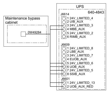
Route the signal cables down through the cable channel in the right side of the UPS and into the maintenance bypass cabinet through the cable entry opening.
