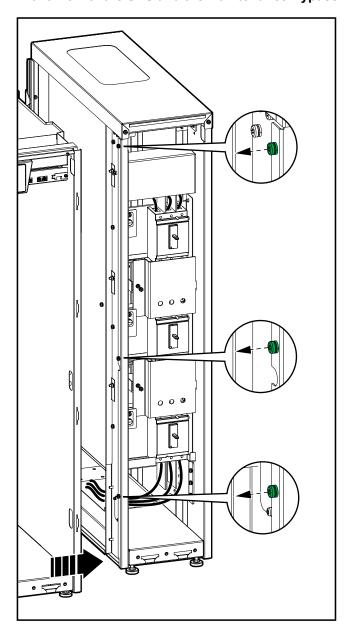
5. Position the UPS close to the maintenance bypass cabinet with a little free space between the cabinets.
