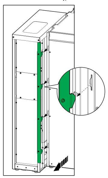
7. Install the three interconnection screws between the UPS and the maintenance bypass cabinet as shown.
