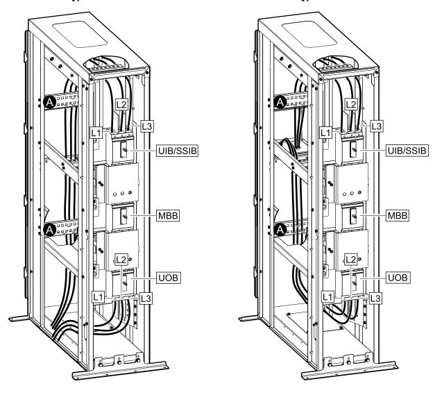
Connect the provided UPS output cables to the unit output breaker UOB (L1, L2, L3) and route the cables out through the left side or through the rear of the maintenance bypass cabinet.
