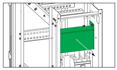
6. Only for bottom cable entry in 100-150 kW maintenance bypass cabinet: Remove the indicated busbars and insulators in the maintenance bypass cabinet for more cable routing space.
