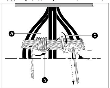
3. Wrap rope (a) several times until the space between the second and the third set of cables is completely filled. Wave the final rope loop (b) underneath the previous loop as shown. Pull the rope taut.
