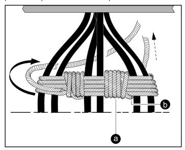
4. Tie rope End 1 and End 2 together as shown. The rope must be taut. Cut off excess rope and tape ends to prevent fraying.
