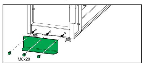
5. Push the maintenance bypass cabinet into position so the rear anchoring bracket connects to the rear anchor. The front anchoring bracket is installed in the final installation steps.
