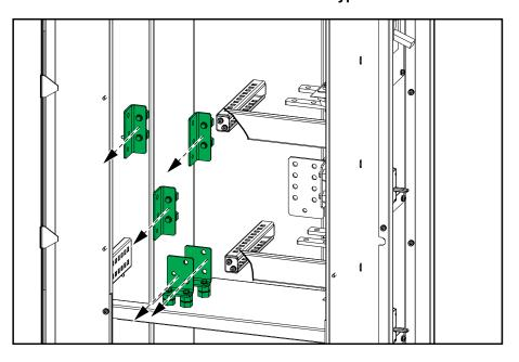
7. Remove the right side panel from the UPS and reinstall the side panel on the right side of the maintenance bypass cabinet. For installation with a UPS for internal batteries, install the 10 supports (A) from installation kit 0H-1717. Reuse the screws from the UPS.
