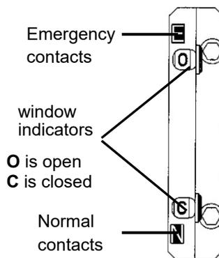
Figure 3. Maintenance handle operation and contact position indicators.
