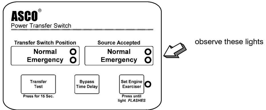
Figure 1-5. Standard controls and indicators.
