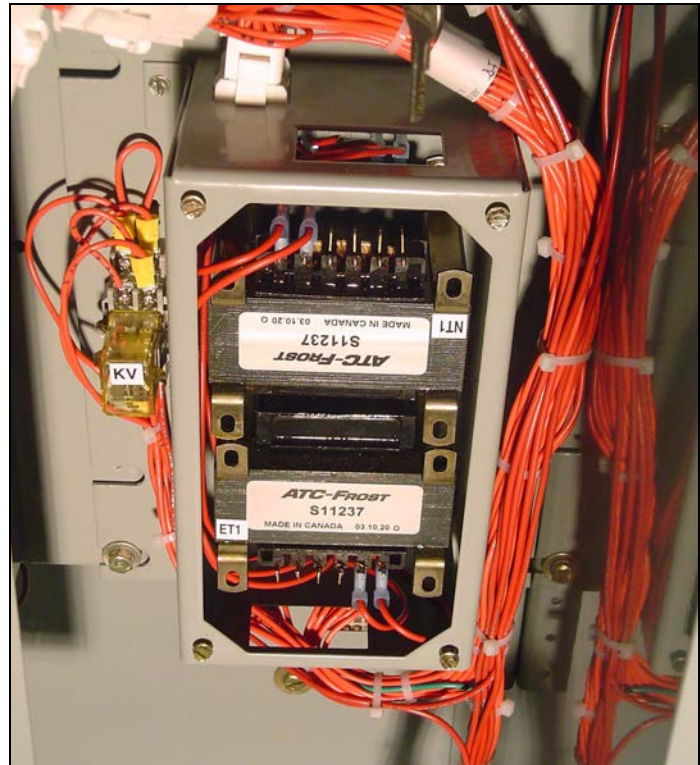
Figure 25. North American Market Voltage Selection Panel with Voltage Being Selected.
