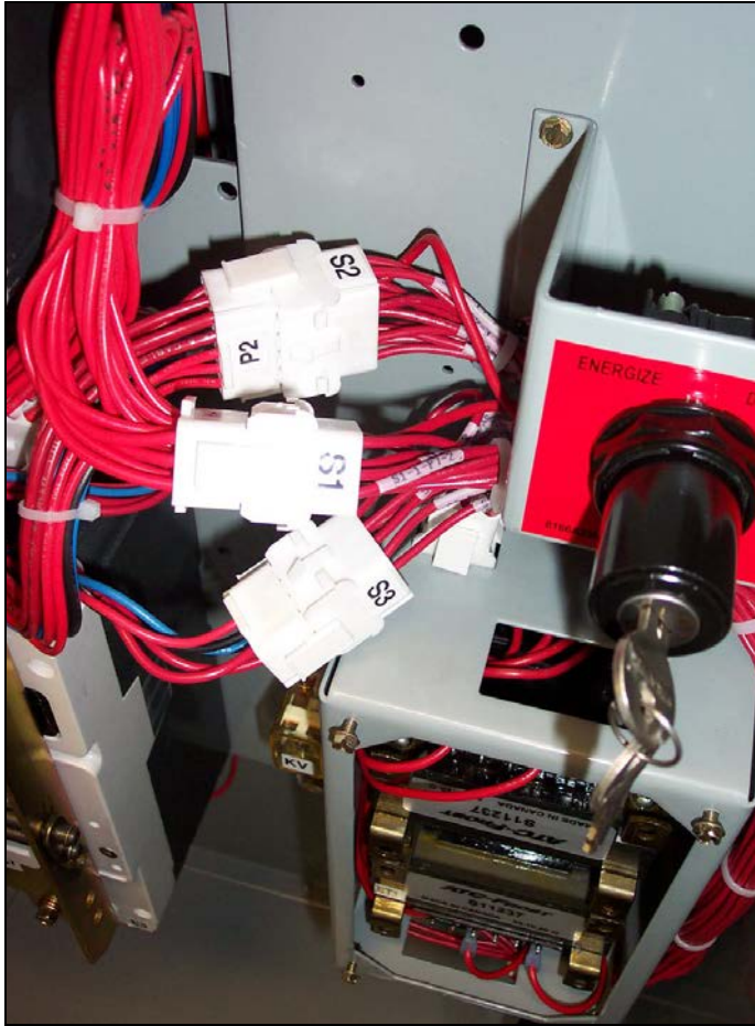
Figure 20. Location of the P1, P2, and P3 Connector Plugs for ATs with the North American Market Transformer Panel.
