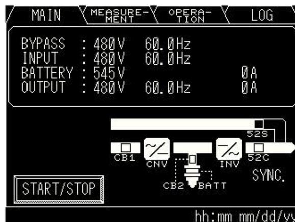
The following will be displayed when the START/STOP key on the MAIN MENU is pressed (Jump into **OPERATION MENU**) :
