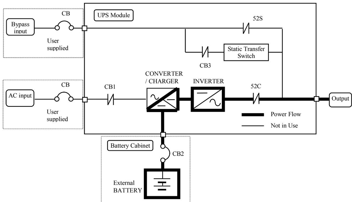
Referring to Figure 1.3: In the event of AC input source failure or interruption, the UPS Converter(s)\* will de-energize and the UPS battery(s)\* will immediately discharge and supply DC power to the Inverter to maintain continuous AC power to the load. This operation will continue until:
