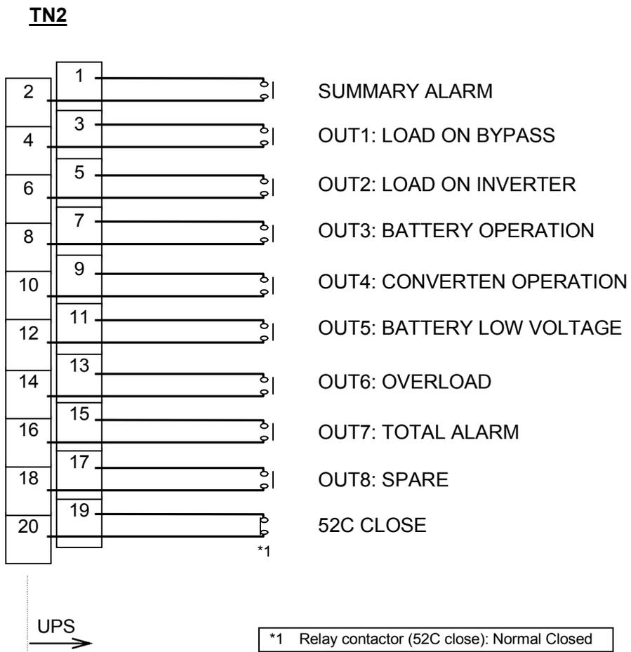
**FIGURE 2.10-b External Signal Terminal Block (NEC Class2)**
