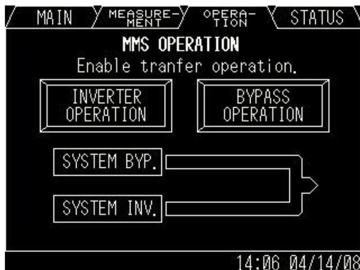
***Transfer from UPS MMS Inverter Operation To UPS MMS Bypass Operation***
