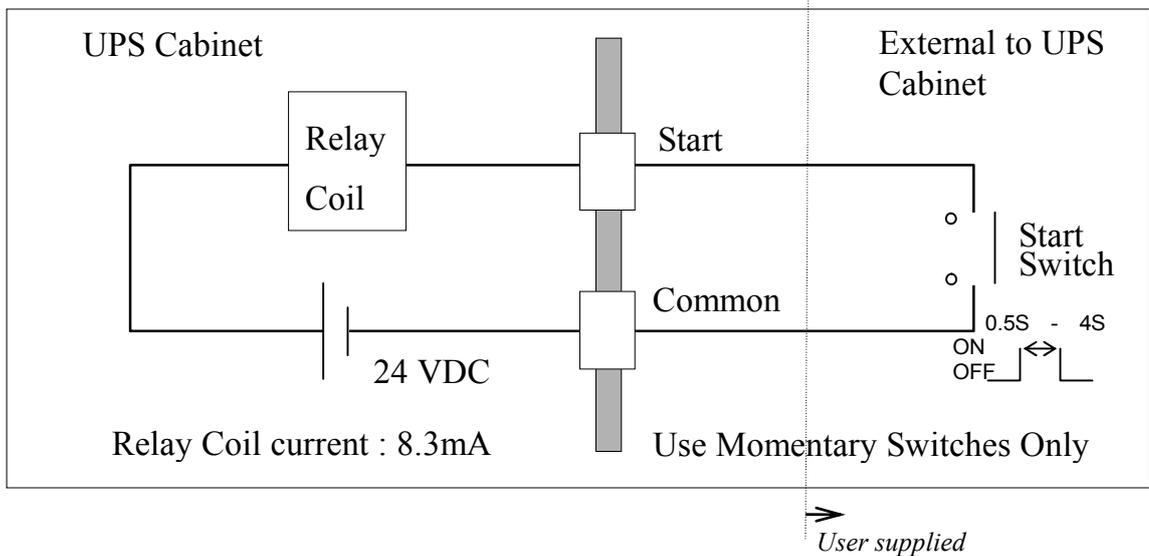
**Details of input contacts for remote access : TN1****Terminals 7 to 8 Remote "Inverter Start" input terminal (IN1)**
