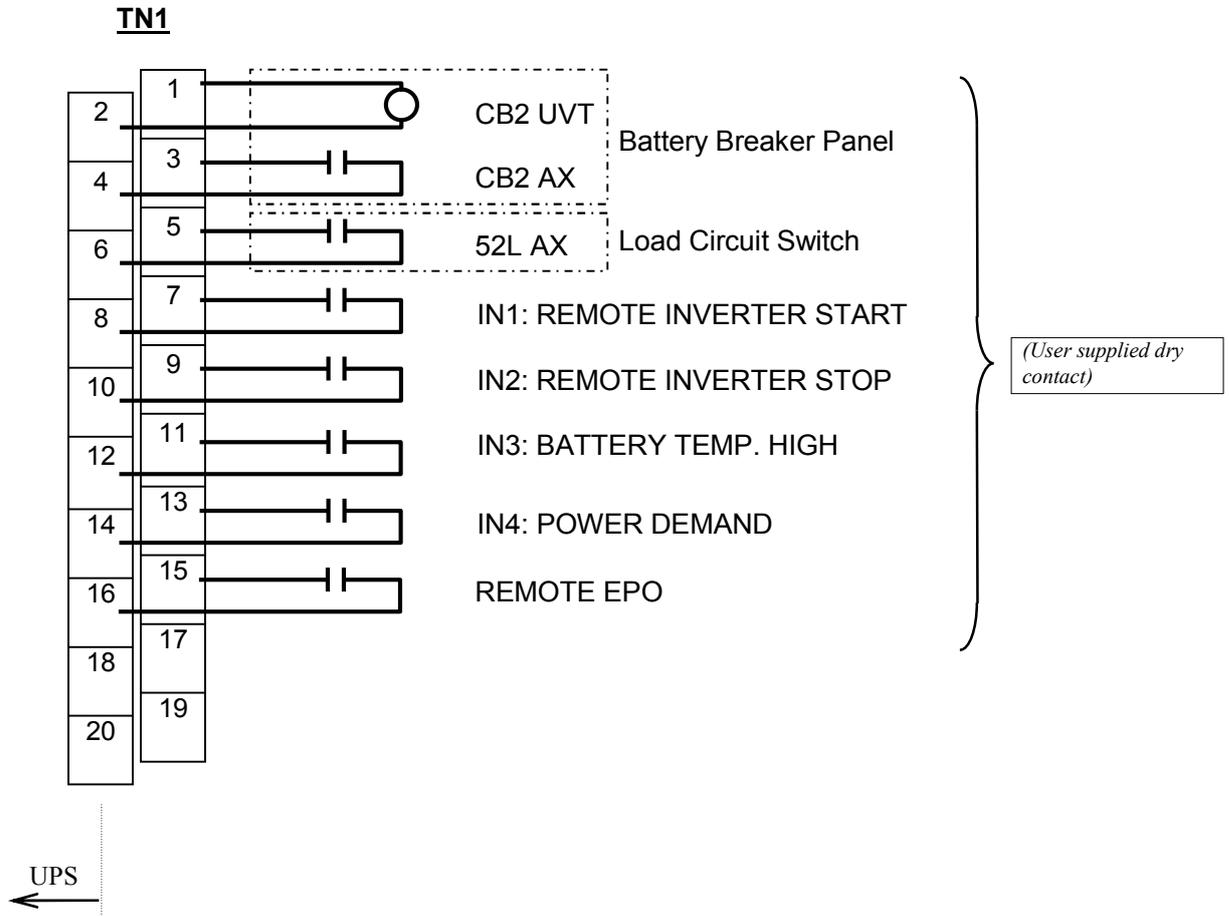
**A) Output Contacts (for external alarm annunciation)**
