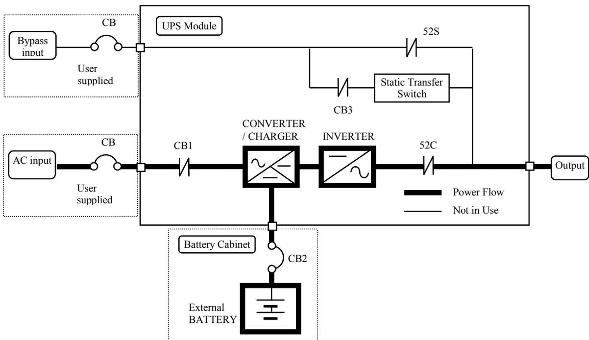
During normal operation, the path through the UPS inverters is used to power the load.
