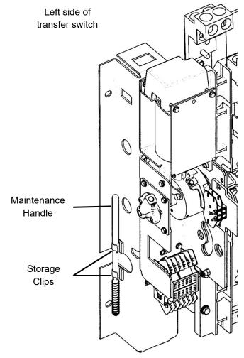
Figure 2 Maintenance handle and its storage clips.
