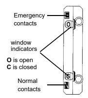
Figure 3. Maintenance handle operation and contact position indicators.
