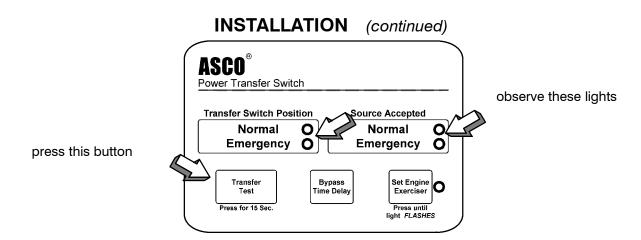
Figure 1-6. Standard controls and indicators.
