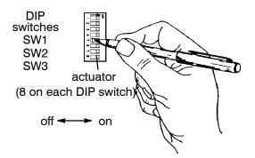
Figure 4-4. Setting DIP switch actuators.
