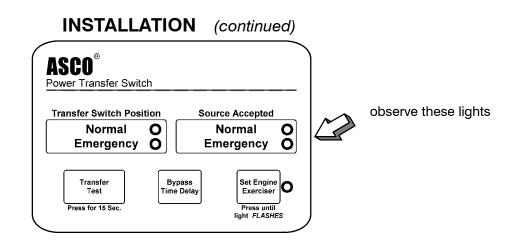
Figure 1-5. Standard controls and indicators.
