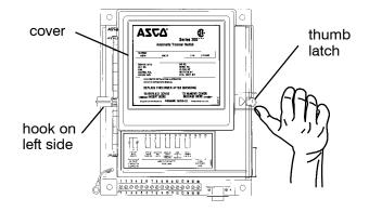
Figure 4-1. Controller cover latch.
