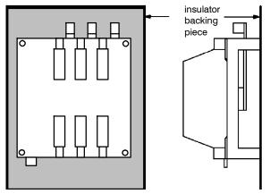
Figure 1-1. Insulator backing piece for 260 and 400 ampere transfer switches.
