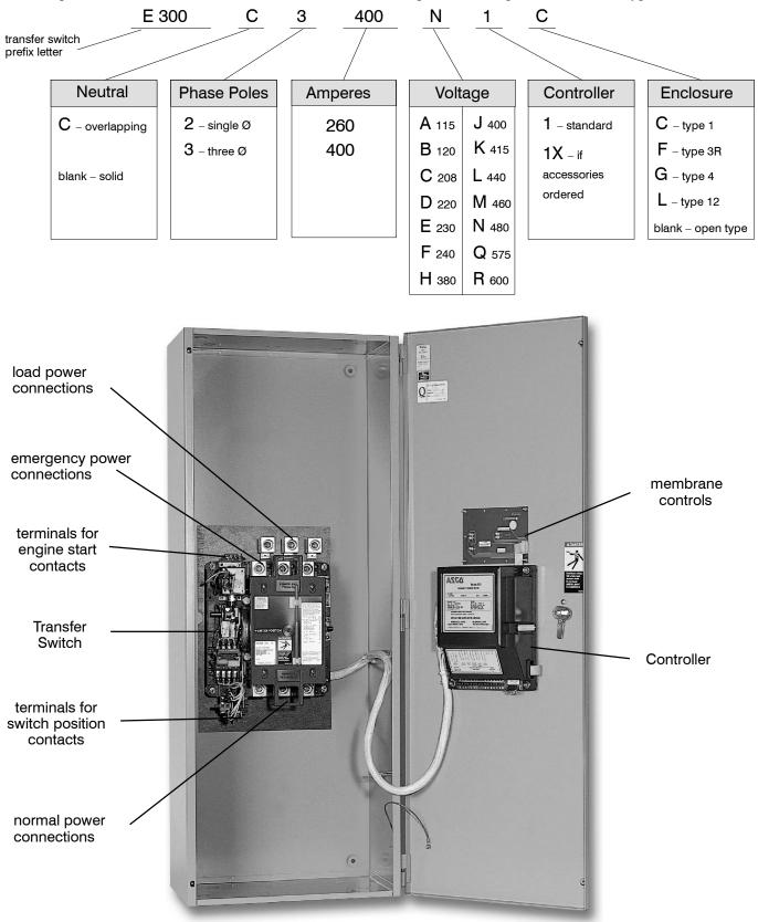
400 ampere size in typical enclosure with location of customer connections
