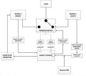
\* A utility voltage monitoring sensor (as shown in the AMF diagram above) must be connected in order to use the AMF feature on the 1302 control. Use Schneider Electric Relay RSB1A120U7 and Socket RSZE1S35M.
