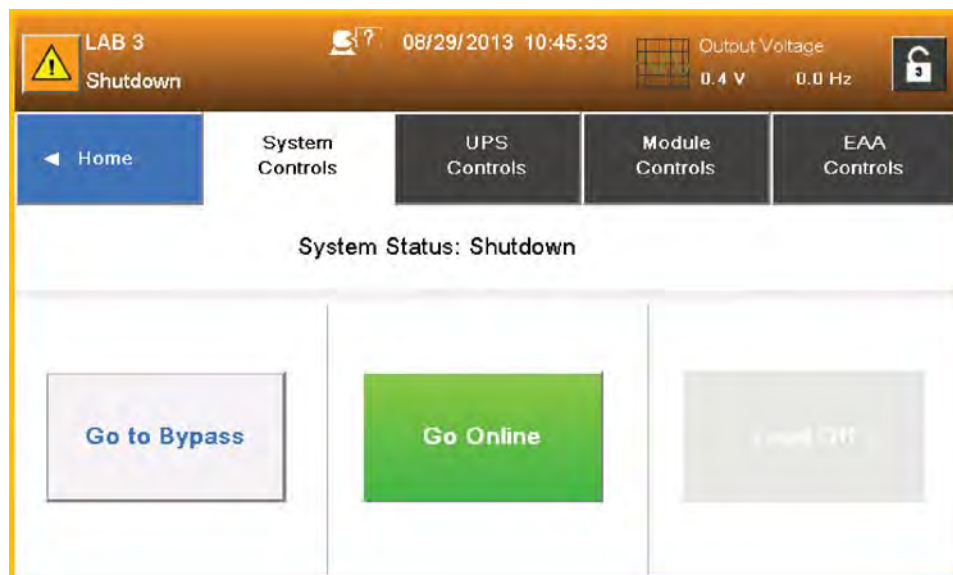
Figure 6-16. Typical System Control Screen
