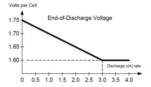
**NOTE:** C equals I<sub>discharge</sub> divided by the battery Ah capacity.
