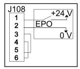
Dry Contacts Normally Closed: EPO is activated when a connection from pin 3 to 5 is opened. Connections: 4-6.
