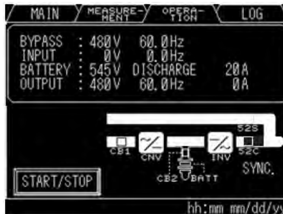
Figure 5-29 Open Battery Breaker
