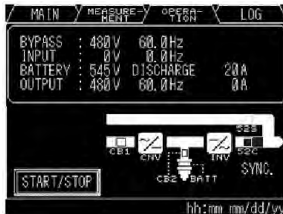
Figure 5-28 UPS Transfers to Bypass
