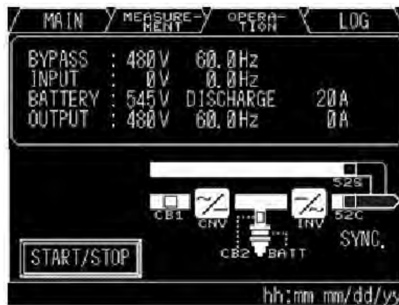
Figure 5-23 Close Battery Breaker
