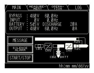
FIGURE 2.7-b Measurement screen (Battery operation)
