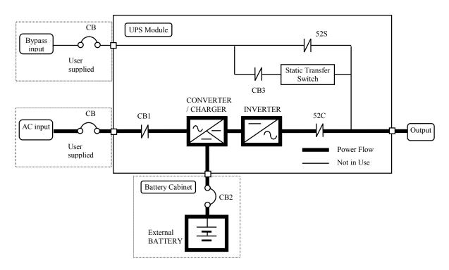
During normal operation, the path through the UPS inverters is used to power the load.
