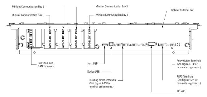
Figure 4-10. Interface Terminal Detail
