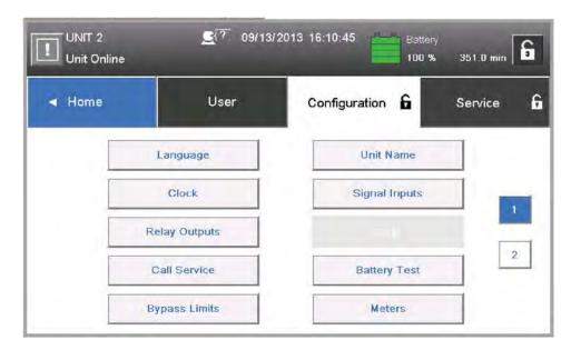
Figure 6-11. Typical Settings Configuration 1 Screen
