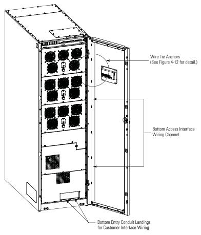
Figure 4-11. Bottom Access Interface Wiring Location
