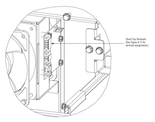
Figure 4-16. Battery Shunt Trip Terminal Detail
