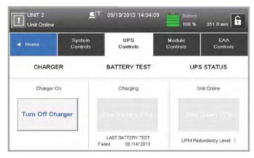
Figure 6-17. Typical UPS Control Screen
