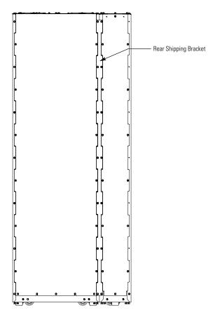
Figure 4-3. Removing the Sidecar Rear Shipping Bracket – Eaton 93PM UPS
