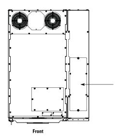
Top Entry Conduit Landing for AC Input and Output, and DC Input (Remove panel to drill or punch conduit holes.)
