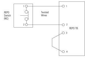
**NOTE** REPO switch rating is 24 Vdc, 1A minimum.
