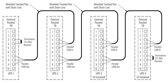
**NOTE 1** External parallel CAN connections between UPS cabinets require shielded twisted pair wire with drain wire.
