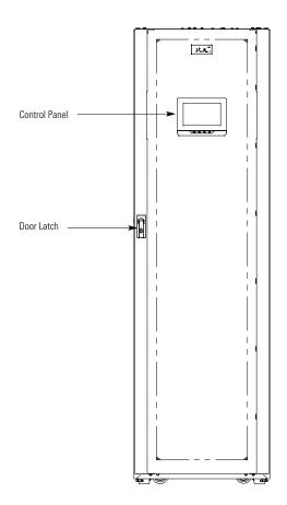
Figure 6-1. UPS Controls and Indicators
