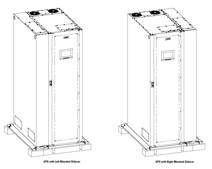
Figure 3-11. UPS Cabinet with Left-Mounted or Right-Mounted Sidecar as Shipped on Pallet
