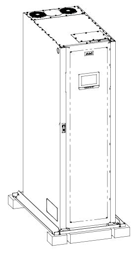
Figure 3-10. UPS Cabinet as Shipped on Pallet
