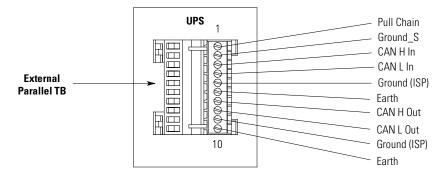
Figure 4-19. External Parallel Terminal Block
