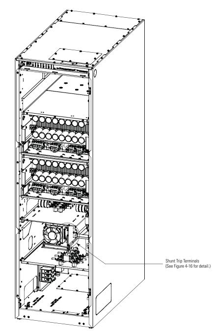
Figure 4-15. Battery Shunt Trip Location
