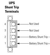
Figure 4-17. Battery Shunt Trip Terminal Assignments
