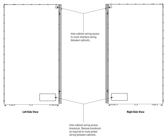
Figure 4-6. UPS Inter-Cabinet Wiring Access Location
