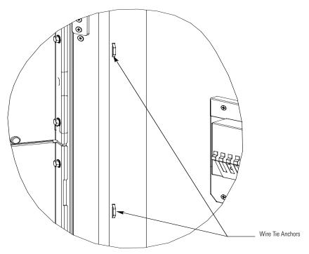
Figure 4-12. Wire Tie Anchors
