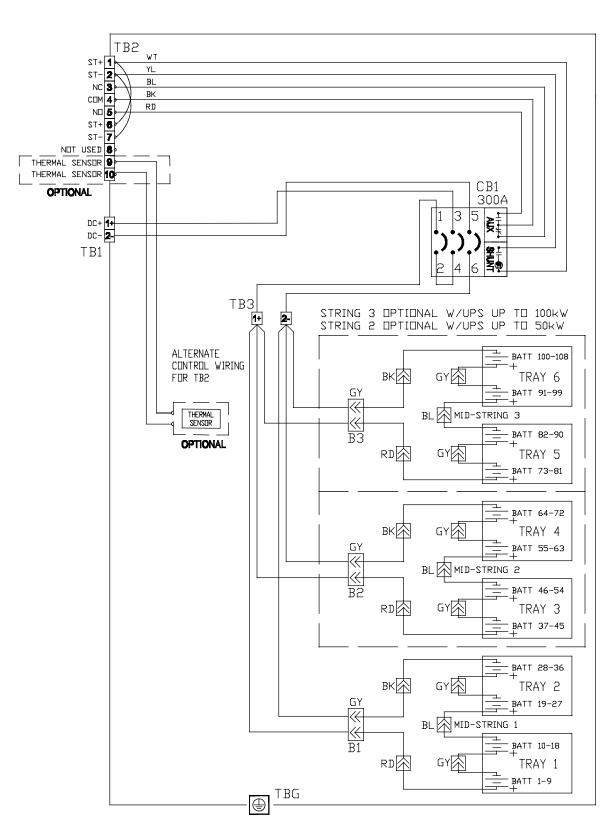
Figure 25. 93PM Integrated Battery Cabinet Schematic
