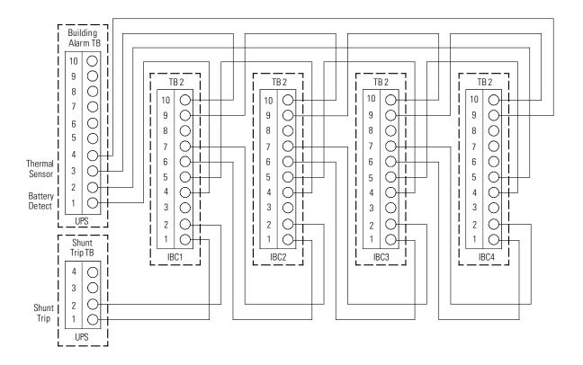
Figure 20. Interface Terminal Detail – Eaton 93PM Integrated Battery Cabinet-Small
