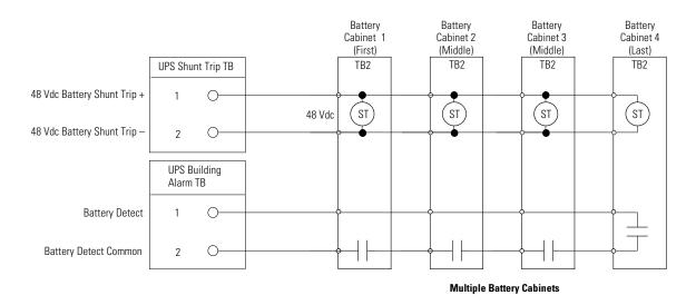
**NOTE** Battery Detect and DC Shunt Trip wiring should be a minimum of 18 AWG.
