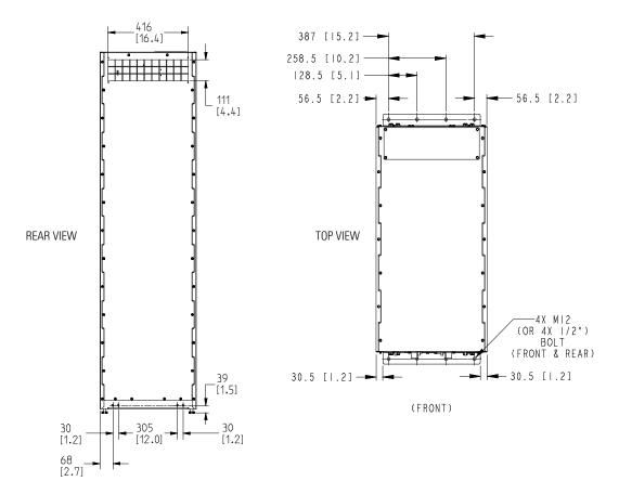
Figure 5. Integrated Battery Cabinet-Small Floor Mount Bracket Dimensions
