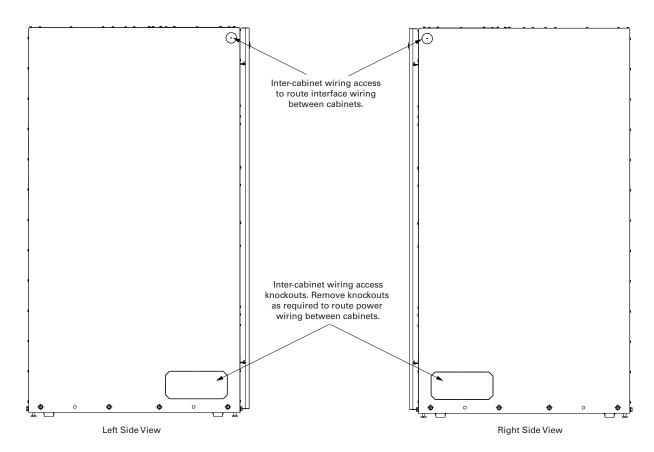
Figure 10. Line-Up-and-Match Wiring Access Locations
