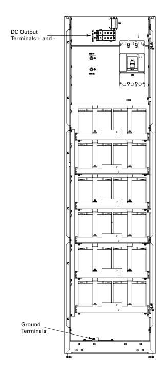
Figure 14. DC Power Terminal Locations – Eaton 93PM Integrated Battery Cabinet-Small
