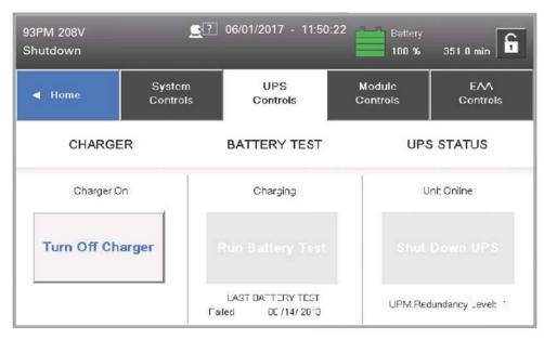
Figure 6-17. Typical UPS Control Screen
